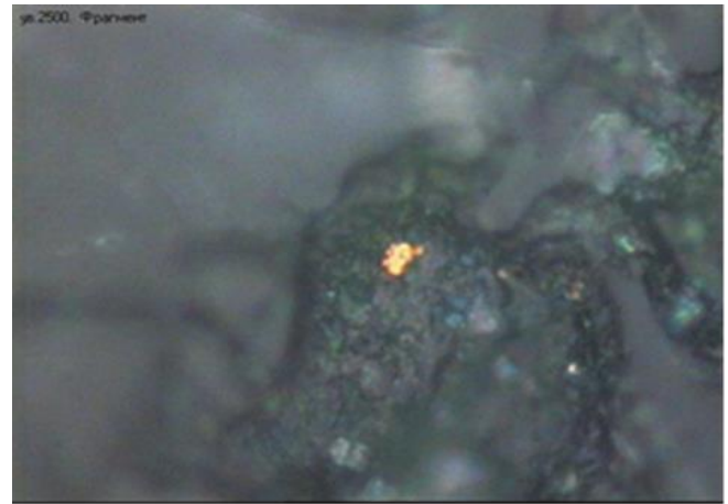
Fig. 6-7. Anschliff 3A- 15, Zengibobo. Increase 500x and 2500h. In the recesses of the fracture zones of quartz, the wrong gold grain size is 0.002mm. The presence of rare gold grains of 0.002mm in indentations of quartz grains has been detected. The quartz aggregates of the granule structure, the quartz grain are subparallel to the dispersion of the containing rocks, bearing signs of fragile deformation.
