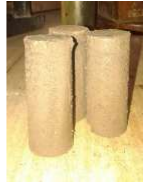
Fig.5 Triaxial test sample
