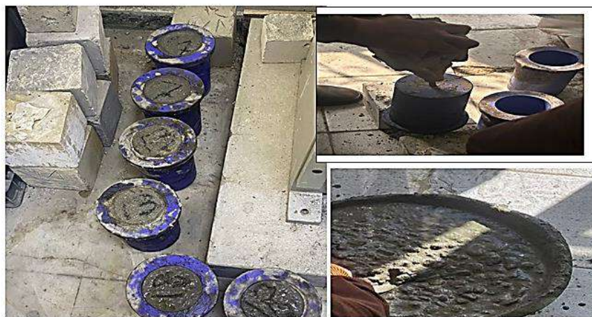
Figure 2. The Mixture of Concrete and the Mold
