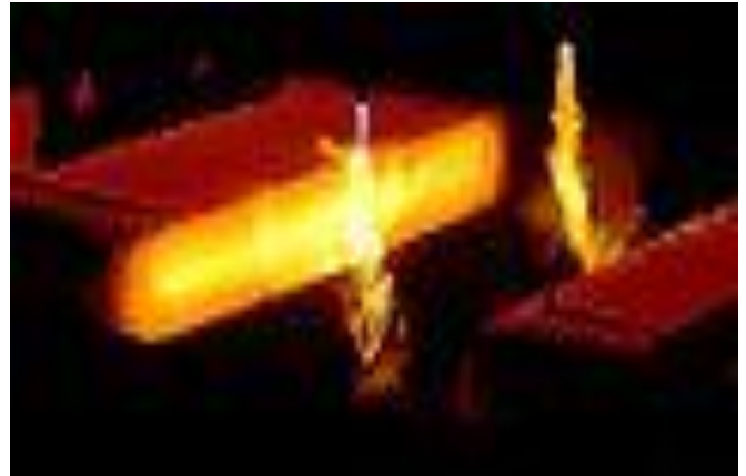
Fig 7.4 oxygen gas torch cutting a slab
