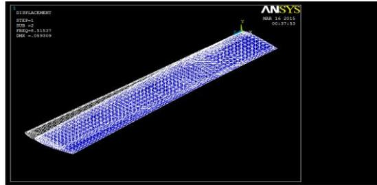
**Fig:13 Modal Analysis of NACA 0015 in 2<sup>nd</sup> Mode of Carbon Epoxy**
