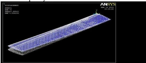
**Fig:12 Modal Analysis of NACA 0015 in 1<sup>st</sup> Mode of Carbon Epoxy**
