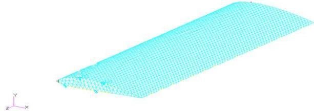
**Fig: 5 Meshed view NACA 23015**
