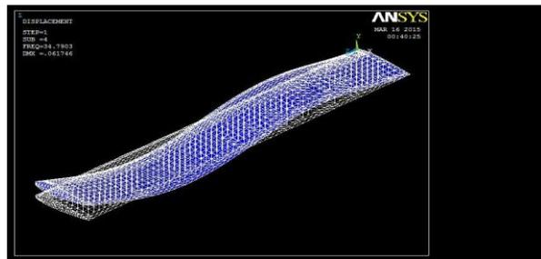
**Fig:15 Modal Analysis of NACA 0015 in 4<sup>th</sup> Mode of Carbon Epoxy**
