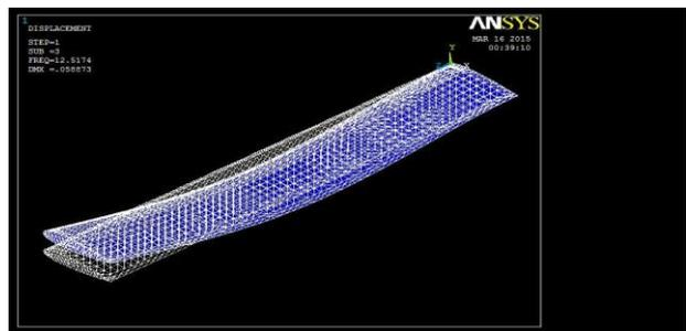
**Fig:14 Modal Analysis of NACA 0015 in 3<sup>rd</sup> Mode of Carbon Epoxy**
