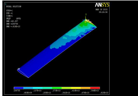
**Fig: 8 Static Analysis of NACA 0015 of Aluminium**
