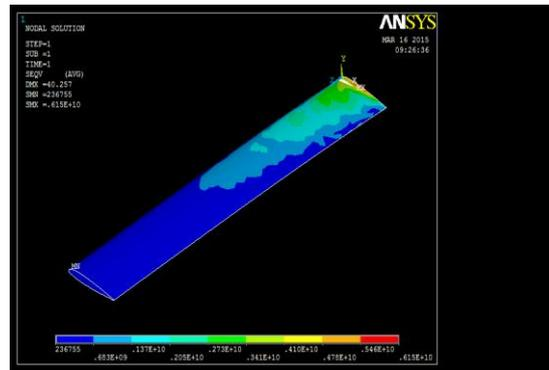
**Fig: 10 Static Analysis of NACA 23015 of boron epoxy**
