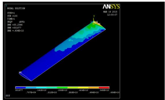
**Fig: 9 Static Analysis of NACA 23015 of carbon epoxy**
