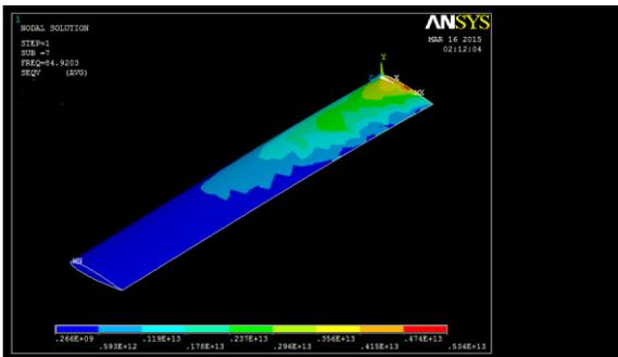
**Fig: 6 Static Analysis of NACA 0015 of carbon epoxy**
