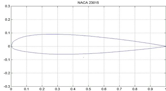
**Fig 2: Airfoil Geometry of NACA 23015**
