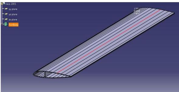
**Fig: 4 CATIA Model of Modified cross section of NACA 23015**
