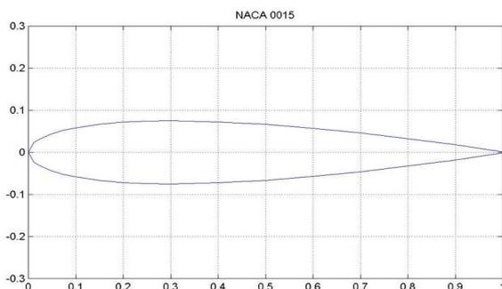
**Fig 1: Airfoil Geometry of NACA 0015**
