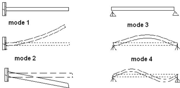
**Fig: 11 Description of Various modes used in Analysis.**
