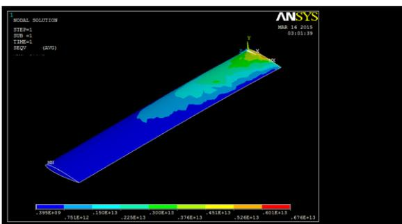
**Fig: 7 Static Analysis of NACA 0015 of boron epoxy**
