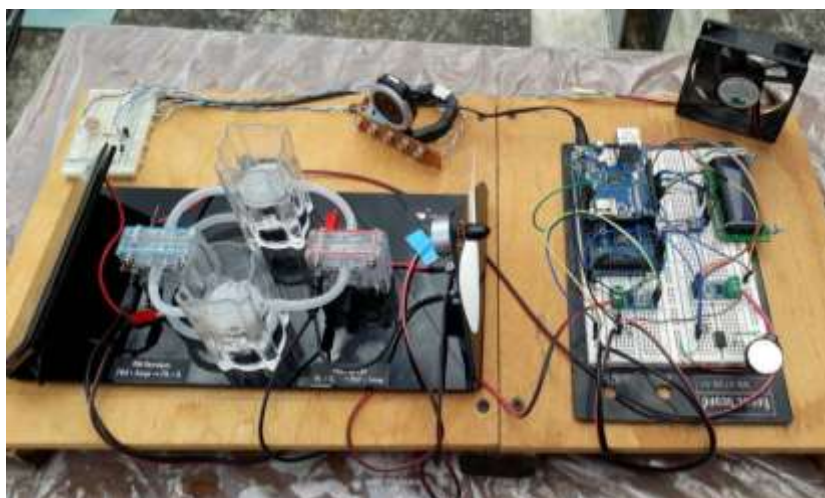
Figure 19: System Hybrid composed of fuel cell and solar PV setup
