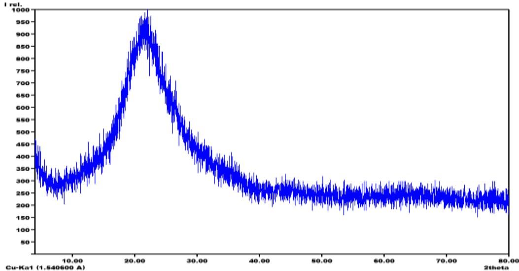
Figure 1. X-ray pattern of microsilica—a waste product of the production of ferroalloy JSC “Uzmetkombinat”
