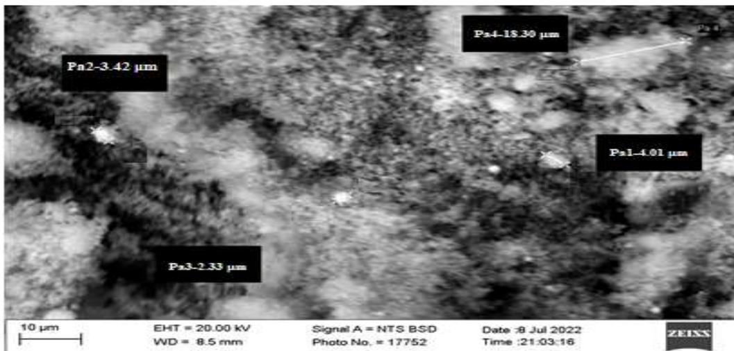
**Figure 2.** The electron microscopic images of microsilica
