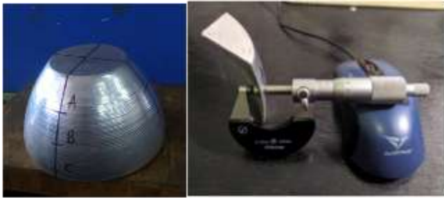
Figure 3. Thickness measurement of the spinning result.
