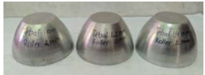
Figure 5. A photograph of the bowl produced by the metal spinning for a 2 mm roller
