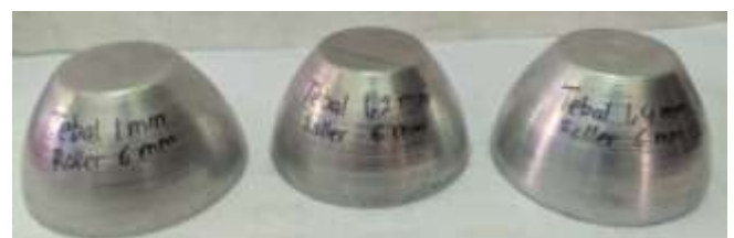
Figure 7. A photograph of the bowl produced by the metal spinning for a 6 mm roller
