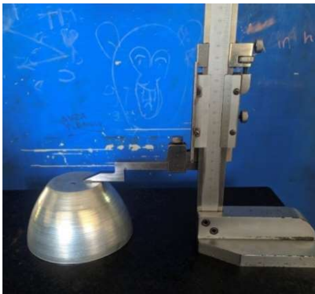
Figure 4. Measurement of the height of the spinning result.
