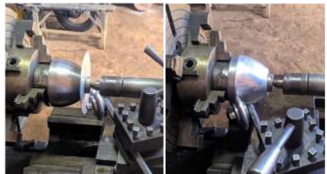
Figure 2. Metal spinning process on a lathe
