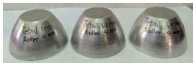
Figure 6. A photograph of the bowl produced by the metal spinning for a 4 mm roller
