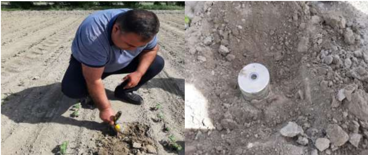
Figure 2. Determination of soil density. The density of the soil between the rows of cotton (between 0–15 cm layers)
