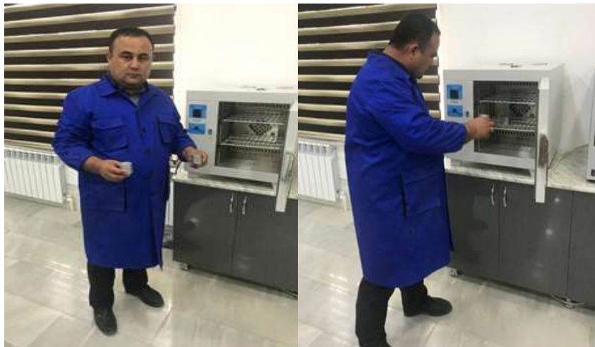
Figure 3. Determination of soil moisture by thermostatic drying
