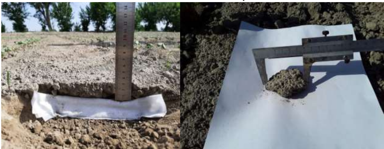
Figure 5. The thickness of the skin was determined with an accuracy of \pm 0.1 cm using a ruler and a caliper
