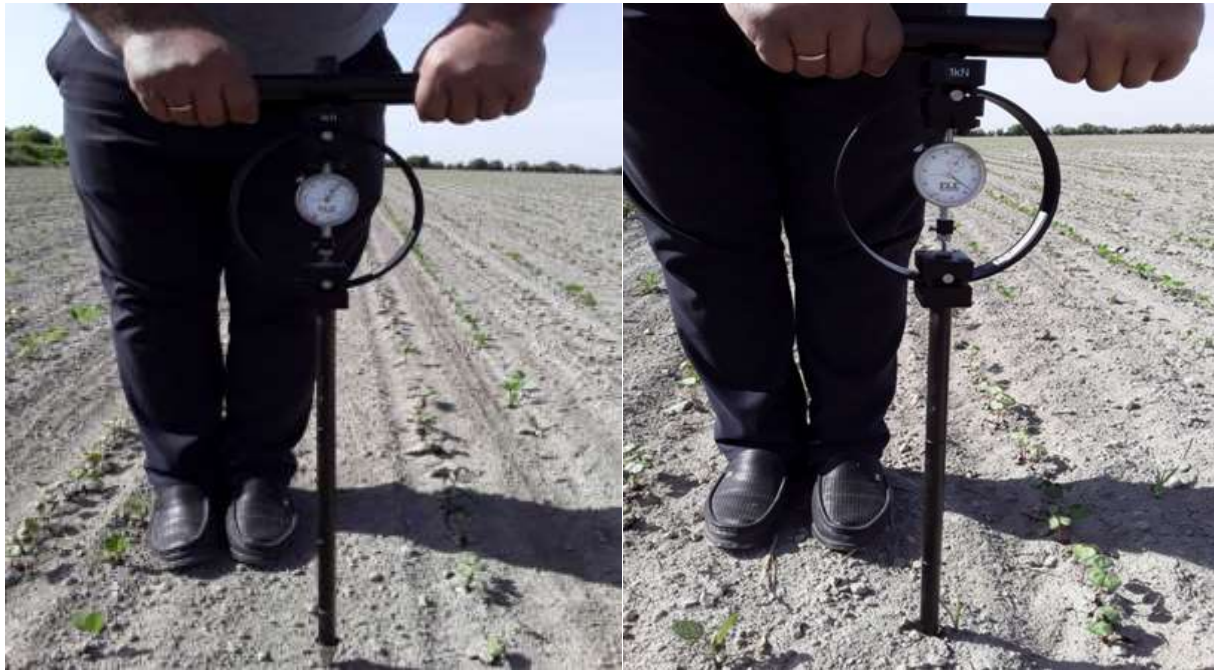
Unimmersed state of the hardometer tool
